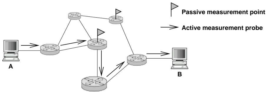
Figure 2: Example of active and passive measurements.
