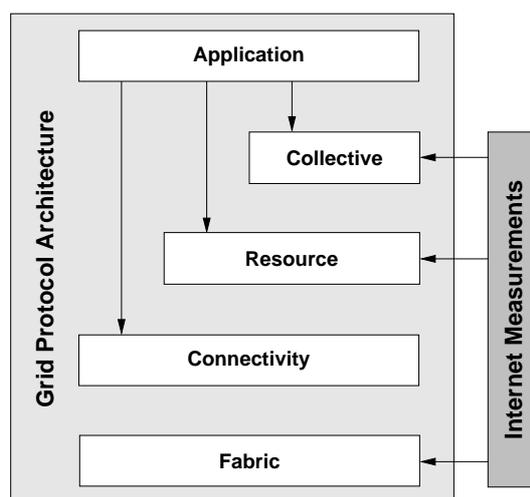
Figure 1: Contribution of Internet measurements to grid layers.
